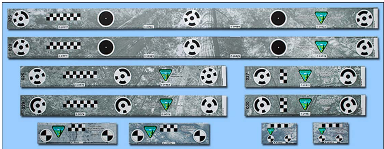
Figure 3 Example of a code bar with targets and rich gray scale background for efficient 3D reconstruction [16].
